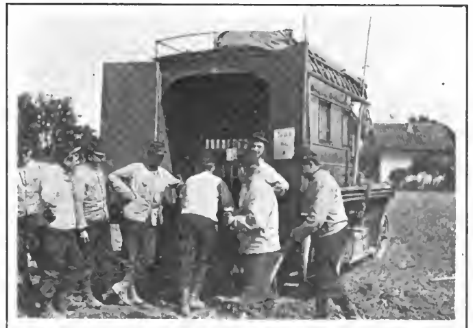
Traveling work shop connected with the aeroplane corps. This is a gasoline truck with a van body containing a dynamo, lathe, drills, band saws, a forge, etc., for repairing aeroplanes
